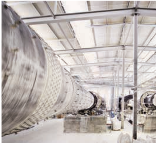
Rotary kiln for calcination of basic NABALOX® grades.
