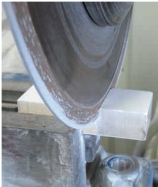
Green machining (cutting) of compacted GRANALOX ® .
